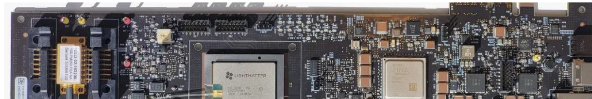
Silicon nano-photonic ANN accelerator prototype from Y. Shen et al., Nature Photonics, 2017
